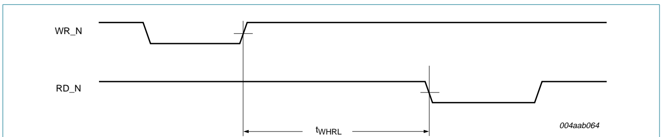
Fig 17. ISP1582 ready signal timing
